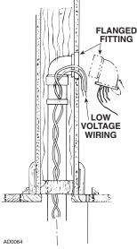
Remove plaster frame from mounting bracket. Pull low voltage wire through hole in bracket and insert bracket into cutout. Secure bracket to flanged fitting with 4 screws provided. Be sure seal is secure between flange fitting and mounting bracket (see figure below).
