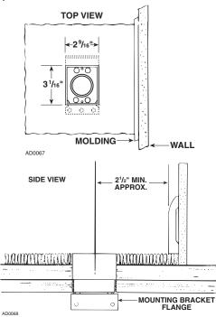
Determine direction of tubing and attach appropriate flanged fitting to mounting bracket with four (4) screws supplied. Be sure mounting bracket flange does not interfere with tubing and seal is securely in place.
