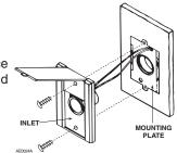
**NOTE**: When wall inlets are installed in walls that are less than 1/2" thick or when inlets are installed back-to-back in a wall, the tube of the wall inlet may extend into elbow area of the flanged fitting and cause blockage. Shorten the wall inlet tube to prevent this condition. Refer to figure below.
