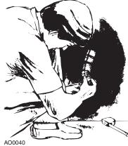
Hold the assembly in place for a few minutes as the cement sets; allow 5 minutes for the cement to completely dry.
