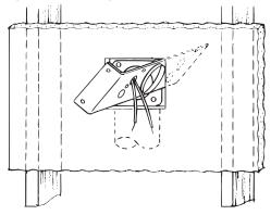
Attach the low voltage wires to terminal screws on back of wall inlet (see figure at right). If using 361 Rough-in with Cl370 Series Inlets, refer to instructions on page 7, step 3, shown in its figure.
