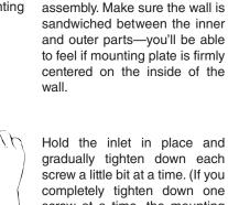
gradually tighten down each screw a little bit at a time. (If you completely tighten down one screw at a time, the mounting plate may pull away from the wall at the loose end and slip back into the cutout.)
