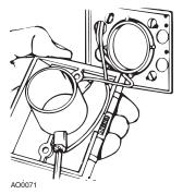
Insert wall inlet into bracket and secure with the two-screws provided (see figure at right).
