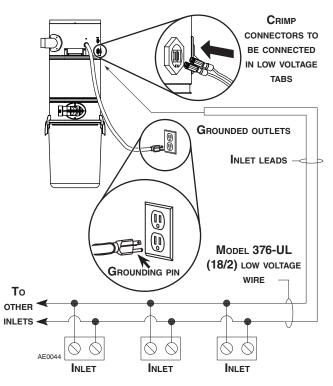
NOTE: Inlet leads to be connected to power unit low voltage tabs using crimp connectors (included in parts bag) and low voltage harness.
