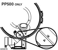
**6 PP500 only:** Put back in place the bag by grasping the edges of its collar and insert over bag adapter. Be careful not to tear the bag. Ensure the collar is positioned between the taper ring and the bag stopper on the bag adapter.
