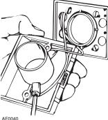
• Cut a 2½" diameter hole in sole plate, header or stud directly in line with opening of inlet bracket fitting. See figure below for center line dimensions.
