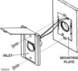
**NOTE:** If CF382S shorter radius elbow is used, it may be necessary to use the short mounting screw to avoid interference with elbow.
