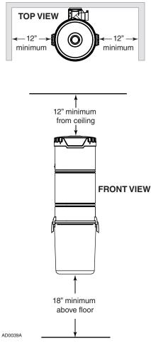
• Position and install the wall mounting bracket with the provided screws. Refer to illustration at right for proper mounting dimensions.
