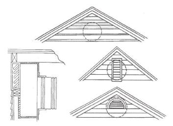
Louvers that are smaller than the ventilator outlet will restrict air delivery. When this condition exists, a chamber should be built to properly direct the air through the louvers. A typical example of the suggested construction is shown.
