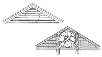
On large triangular louvers, mount to the frame or nail boards to the frame to provide a mounting surface for the ventilator.
